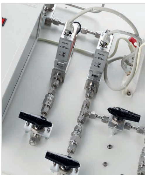
High precision mass flow controllers (MFC) and intelligent gas dosing and pressure system of a Linseis STA HP L84 guarantee optimum performance under various conditions in the full pressure and temperature range
