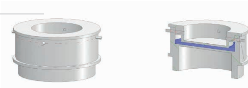
Sample holder for liquids and pastes
