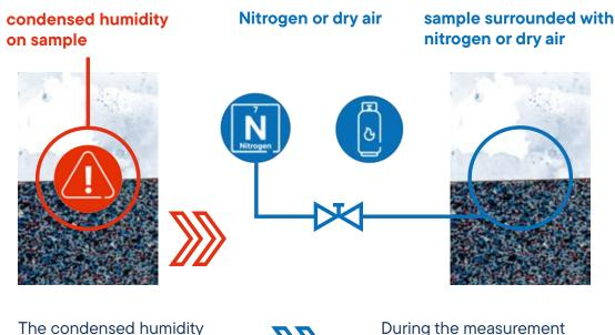
The condensed humidity (dew) might be soaked into the sample and change the thermal conductivity of the sample.
