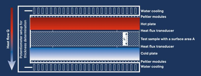
Fourier's law of heat conduction is the basis for the calculation of thermal conductivity and thermal resistance.
