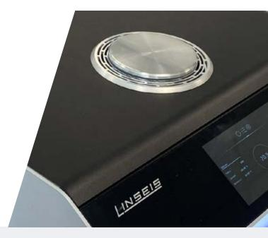
The LINSEIS Differential Scanning Calorimeters (DSC) operate in agreement with national and international standards such as: ASTM C 351, D 3417, D 3418, D 3895, D 4565, E 793, E 794, DIN 51004, 51007, 53765, 65467, DIN EN 728, ISO 10837, 11357, 11409
