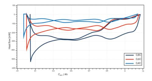
Heat flow over the capacity of a 1-cell Li-ion standard battery at different charge and discharge currents. This allows differences in the efficiency of various charging parameters to be displayed depending on the capacity of a battery. What is striking here, for example, is the different residual capacity depending on the different discharge parameters. A significant increase in heat flow at higher charging and discharging currents is also evident.
