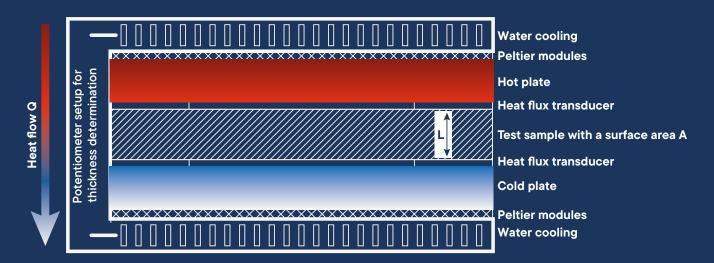
Fourier's law of heat conduction is the basis for the calculation of thermal conductivity and thermal resistance.
