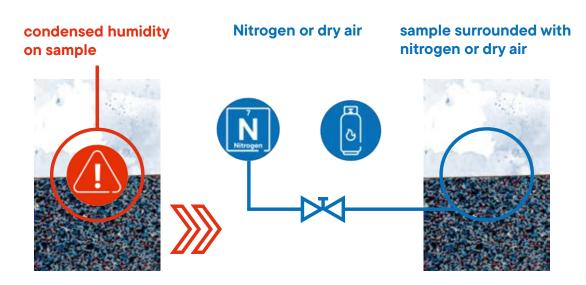
The condensed humidity (dew) might be soaked into the sample and change the thermal conductivity of the sample.
