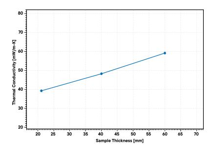
Compressible materials can change their properties depending on the compression. This was demonstrated on a mat of polyester fibers. A sample of size 300 mm x 300 mm and initial thickness of about 60 mm was placed into a Linseis HFM 300 and tested at room temperature.
